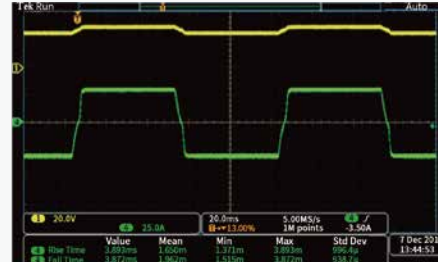
Control loop CC priority mode
